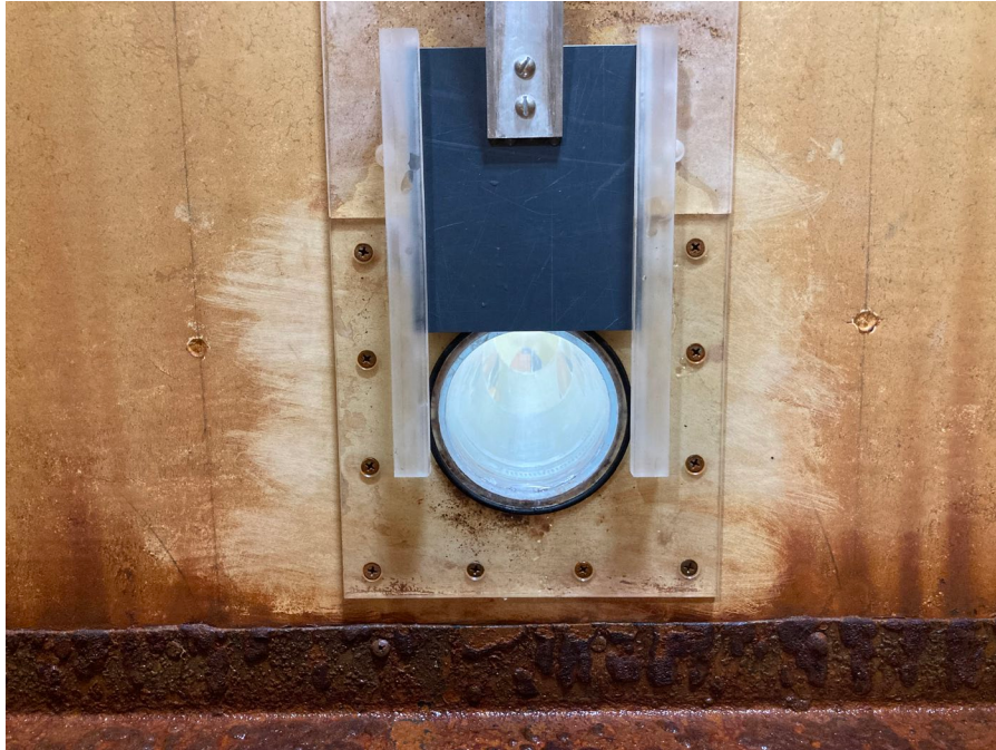
Figure 2.—Photograph of the Clear Creek scaled physical model showing the square shaped gate leaf upstream of the penstock (looking downstream; Kubitschek 2022).
